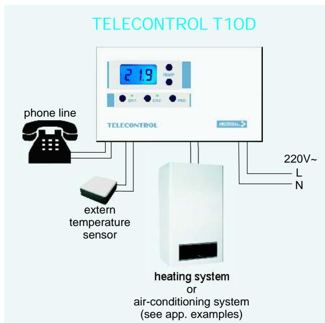
Room thermostat with built-in voice communication interface for remote control via phone or cell phone.
